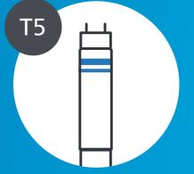
Two rings: HF (High-frequency Electronic ballast)
