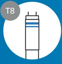
Two rings: HF (High-frequency Electronic ballast)
