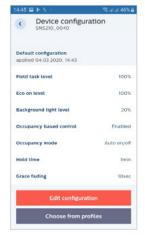
EasySense SNS210 MC parameters can be configured via MasterConnect App.
