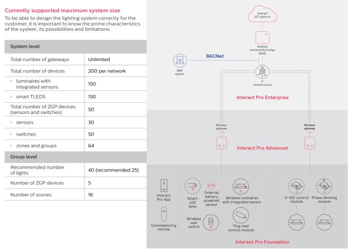
Interact compatible via bluetooth (like SpaceWise) or connected with gateway
