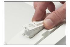
Step 2: Remove the two wires that were secured to the back of the plate and insert them in an approved sensor for use with EvoKit. They are not polarity sensitive.
