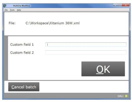
If in the preferences the option **Use custom fields**, **Custom field 1** or **Custom field 2** is checked, MultiOne Workflow will display a window in which one or two custom fields can be filled in. These fields will be stored as part of data logging, together with the generated label data and/or will be printed on a label (depending on the selected options).
