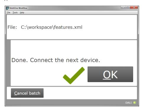
Disconnect the device and connect a new device. Click **OK** to configure the new device. Click **Cancel batch** to go to the main application window.
