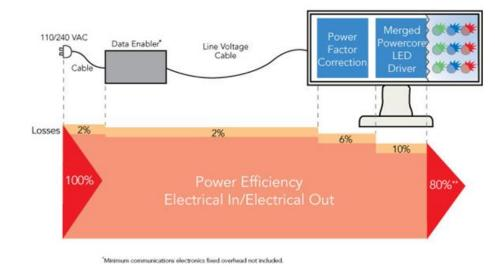
Powercore® is a patented breakthrough in digital power processing technology that surpasses traditional power supply technology by streamlining multiple conversion and regulation stages into a single, flexible, microprocessor-controlled power stage that rapidly, efficiently and accurately controls power output to LED-based systems directly from line voltage, eliminating the need for an external power supply.
