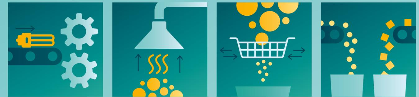
**01** The lamps are fed into a crushing unit, which breaks them into smaller pieces in order to facilitate further treatment and recovery of the various fragments.
