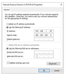
Close the window and save the configuration by clicking the OK tab.
