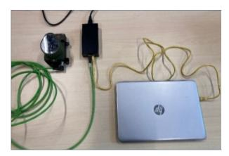
After the configuration of the Trulifi 6014 units is completed, the system is ready to be installed. Note that the optimum performance of the LiFi link can only be achieved when the Access Points and End Points are perfectly aligned. To support this alignment, there are various mounts as well as a laser pointer available as options which are sold separately.
