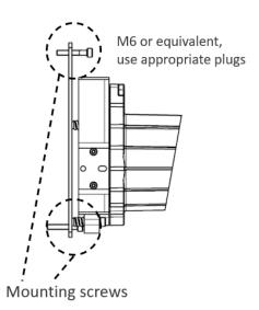
After device is correctly mounted and connected (see chapter 6.3) with a hex key (not provided) the fine adjustment screws can be used to optimize the connection.
