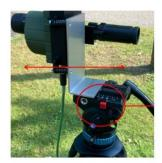
Latch to attached and remove the Trulifi 6016 from the base of the tripod
