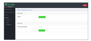
When using the factory reset option, all system configuration settings will be lost, and the device will return to the Long Range Mode / LEDs ON.
