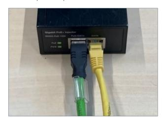
ii. When correctly powered the following ALL LEDs will start to illuminate for about 3 seconds, after which some LEDs will extinguish
