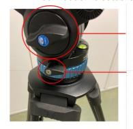
Tighten or untighten this knob to disable/enable vertical adjustment of the unit
