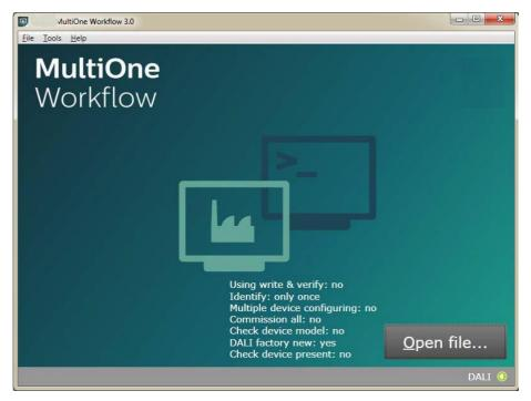
Feature file and schedule file are both Workflow files. If the **DALI protocol** is used and the configuration mode is **Single shot**, then Workflow accepts both type of Workflow files. Otherwise, Workflow will only accept feature files. To open a file, select **File**  $\rightarrow$  **Open...** or click **Open file**. Select a file and click **Open**.
