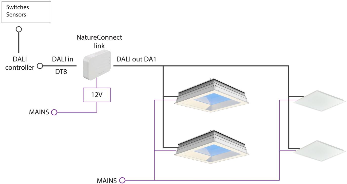
NatureConnect link makes use of a DALI CCT value, coming from the DALI controller, to enable the “Dim to warm” dynamic behaviour. The colour temperature of the luminaire is related to the brightness level. With the maximum light output the light is cold, when dimming to lower values, the colour temperature is warmer.
