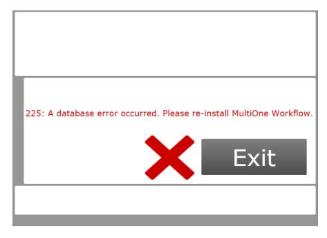
Click **Exit** to close the application window and re-install the MultiOne Workflow.
