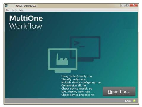
Feature file and schedule file are both Workflow files. If the **DALI protocol** is used and the configuration mode is **Single shot**, then Workflow accepts both type of Workflow files. Otherwise, Workflow will only accept feature files. To open a file, select **File** → **Open...** or click **Open file**. Select a file and click **Open**.
