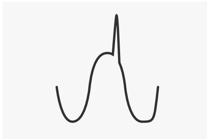
Figure 1: Transient "surge" overvoltage
