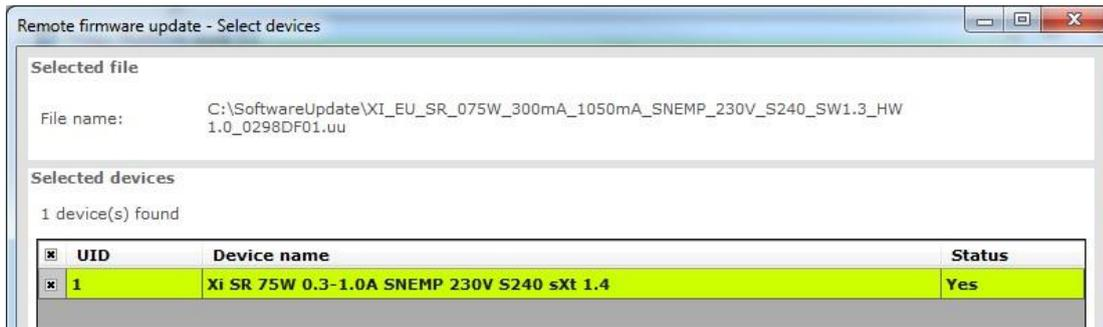
All supported devices for this update procedure are retrieved and listed. The status column describes the reason why a device is or isn't supported. The user can select the devices from the list and when one or more supported devices are selected the user can press **Start** to start the remote firmware update. During the update, the user can see the progress status, the different stages of the update and is able to abort the update procedure.
