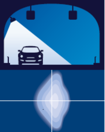
Typical 2-lane tunnel/cornice configuration
