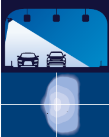
Typical 3-lane tunnel/cornice configuration
