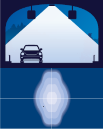
Typical 2-lane tunnel/central configuration
