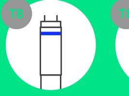
One ring: EM/Mains (Electro-magnetic ballast or direct mains)
