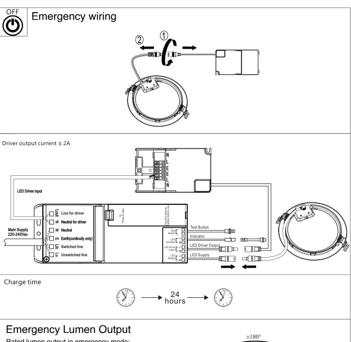
Rated lumen output in emergency mode: DN145B LED6S/830\_840 WH: min 270lm DN145B LED10S/830\_840 WH: min 280lm DN145B LED20S/830\_840 WH: min 290lm
