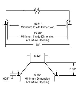
\*\*Please Note: When installing emergency lighting, a greater minimum depth may be required.
