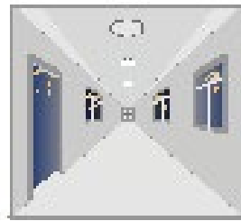
Sensor turns OFF light after standby period.
