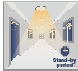
After holdtime, sensor dims light to standby dimming level for standby period. If standby period has been set as 0s, sensor turns light OFF automatically after holdtime.
