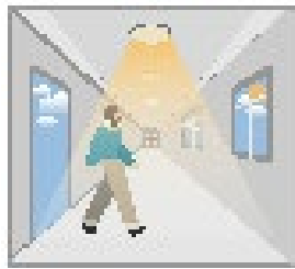
Sensor turns ON light when motion is detected
