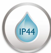
two figures: the first one refers to the protection level against dust, the second against water. This lamp is designed with IP44: it is protected against splashing water. This product is most common and ideal for general outdoor use.
