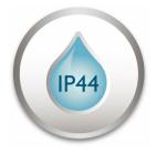
This Philips PIR sensor is especially designed for humid outdoor environments. It was tested rigorously to ensure its water resistance. The IP level is described by two figures: the first one refers to the protection level against dust, the second against water. This Philips PIR sensor is designed with IP44: it is protected against splashing water, ideal for general outdoor use.
