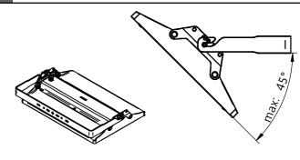
SWP , MSP, CHEM, C4H versions The angle of luminaire position cannot be adjusted after fixation to avoid scratches on painted surface
