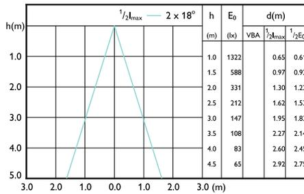
Beam diagram - MASTER LED 6.5-50W 927
