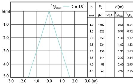
Beam diagram - MASTER LED 6.5-50W 940
