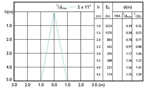
Beam diagram - MAS LEDspotLV D 7.5-50W
