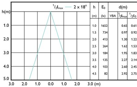
Beam diagram - MAS LEDspotLV D 7.5-50W
