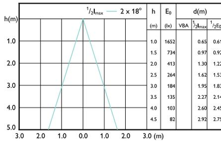
Beam diagram - MAS LEDspotLV D 7.5-50W
