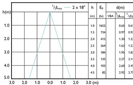
Beam diagram - MAS LEDspotLV D 7.5-50W
