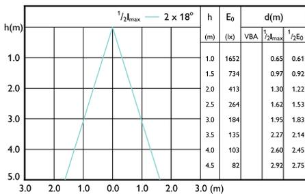
Beam diagram - MAS LEDspotLV D 7.5-50W
