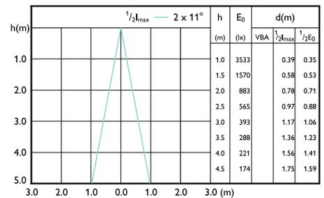
Beam diagram - MAS LEDspotLV D 7.5-50W
