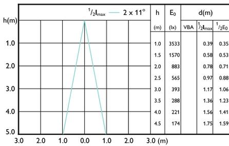
Beam diagram - MAS LEDspotLV D 7.5-50W
