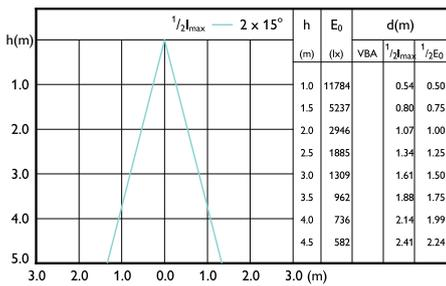
Beam diagram - Master LED PAR30L 28W 30D
