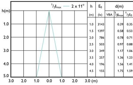
Beam diagram - CorePro LEDspot ND 9-60W
