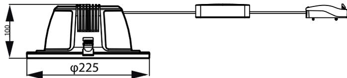
Cut-out hole diameter - Ø200mm
