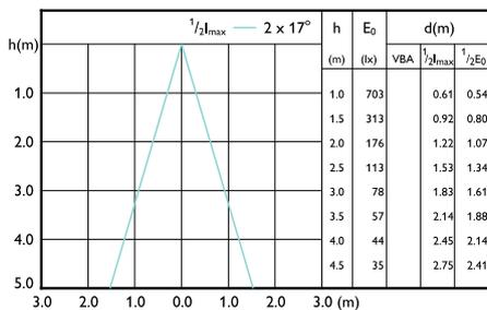
Beam diagram - MAS LEDspot UE 2.1-50W
