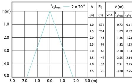
Beam diagram - MAS LEDspot UE 2.1-50W
