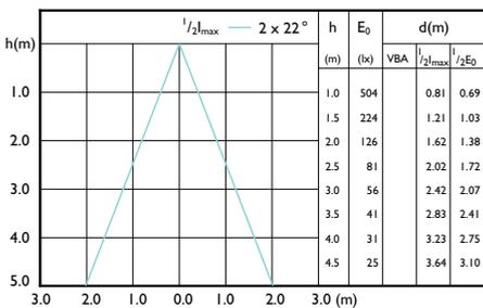
Beam diagram - MAS LEDspot UE 2.1-50W
