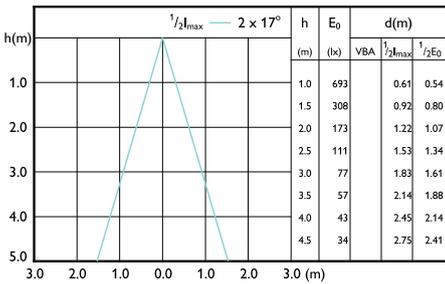
Beam diagram - MAS LEDspot UE 2.1-50W
