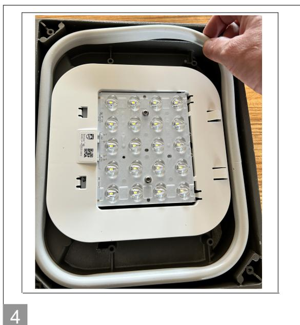
5. Disconnect PCB LED and remove Lensplate and PCB LED
