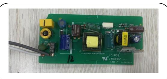
Electrical connection of driver 17W
