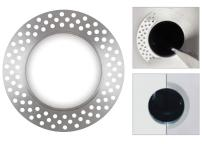
Mud-in ring (FMR): Low profile, non-metallic mudin ring provides a raised rib to plaster up to and a 3/16" flange thickness. The ring is attached to the ceiling material as opposed to the frame-in kit to avoid conduction of heat and vibration which can cause yellowing or cracking of the plaster.
