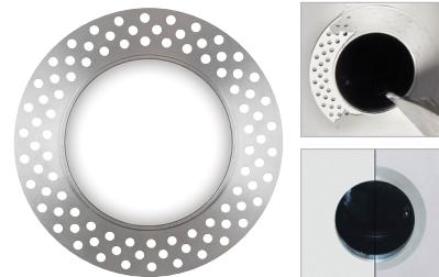
**Mud-in ring (FMR):** Low profile, non-metallic mud-in ring provides a raised rib to plaster up to and a 3/16" flange thickness. The ring is attached to the ceiling material as opposed to the frame-in kit to avoid conduction of heat and vibration which can cause yellowing or cracking of the plaster.
