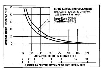
Use quick calculator chart to determine the spacing of 75 Watt PAR30 FL units (Black) for a desired level of illumination. Conversion Factors: 75W PAR30 FL, White, F.C. x 1.1.
