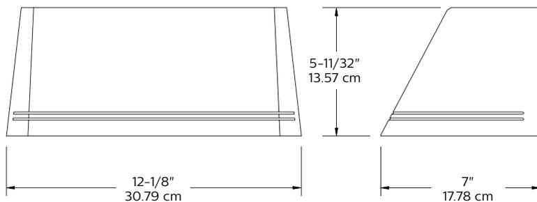
Note: Mounting plate center is located in the center of the luminaire width and 2.38" (6.03cm) above the luminaire bottom (lens down position). Splices must be made in the J-box (by others). Mounting plate must be secured by max. 1/4" (.64cm) diameter bolts (by others) structurally to the wall.
