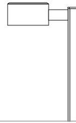
The Gardco arm mounted Square Form 10 products are cutoff luminaires for high intensity discharge lamps up to 400 watts. The EH units are manufactured from mitered extruded aluminum and finished in an Architectural Class 1 anodizing. Can accept one of seven (7) interchangeable and rotatable precision segmented optical systems. Flat glass lens luminaires provide full cutoff performance. Sag Lens luminaires provide cutoff performance.
