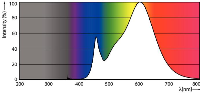
Spectral Power Distribution Colour - LEDBulb 14.5W E27 3000K 230VA67
