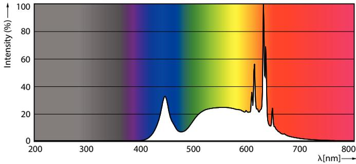
Spectral Power Distribution Colour - CorePro LEDspot 3-35W GU10 840 36D DIM
