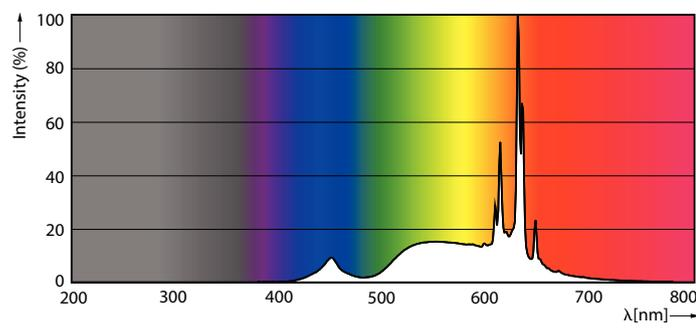
Spectral Power Distribution Colour - MAS VLE LEDBulbDT5.9-60W E27 927A6OCL G
