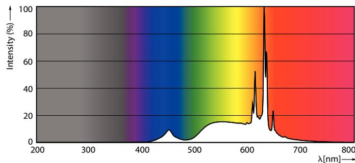
Spectral Power Distribution Colour - MAS VLE LEDBulb DT5.9-60W E27
