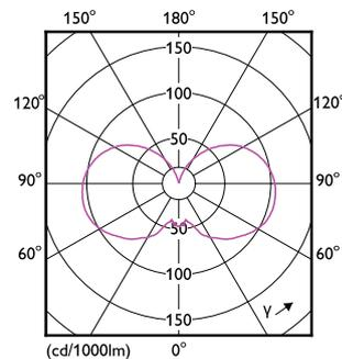
Light Distribution Diagram - MAS VLE LEDBulb DT5.9-60W E27
