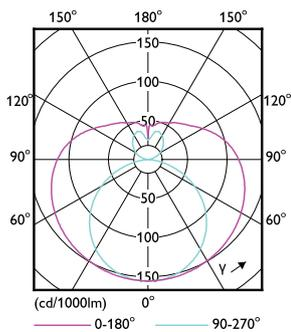
Light Distribution Diagram - CorePro LEDtube 1200mm 14.5W840
