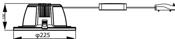
Cut-out hole diameter - Ø200mm
