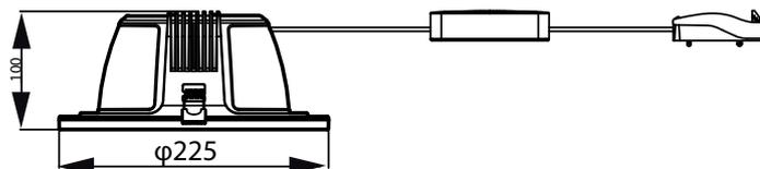
Cut-out hole diameter - Ø200mm
