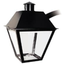
The **L40U** luminaires feature a one-piece square tapered cast aluminum housing, with a sealed optical system. The cast-aluminum hood includes a photoelectrical hiding decorative finial, assembled on the housing using two built-in hood hinges.
