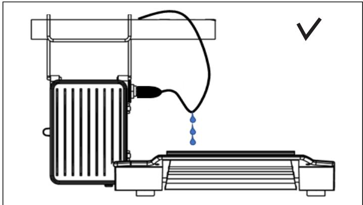
Connect the female connector of the main power cable <CLICK> and connect this main power cable to the power grid. Make sure to relieve the stress from the cable connections, by introducing a loop (see install pictures on the first page).
